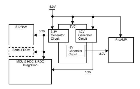
Figure 4.1 Power supply configuration
